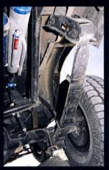
Deaver leaf packs have few peers in the leafspring world, so they were a natural choice for springing the Explorer's tail section. Since an SUV has a heavier tail than a pickup, the spring rate was matched to the application. A spring-under configuration
