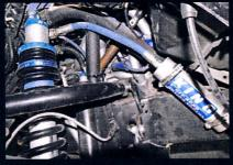
A Peer past the King dampers and the Blitzkrieg metalwork and you'll find a pair of Torque Monster headers bolted to the 5.0. These smog-legal pipes awaken the Ford small-block to the tune of 20 additional ponies and up to 40 lb-ft of added torque. The V8 is a good match for the chassis; it had no problem moving the Explorer through the deep whoops of Ocotillo Wells at high velocity.
