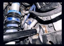
Adjusting caster and camber with the stock eccentric bolts can be a hassle, so Blitzkrieg nixed them altogether in favor of rod ends; the alignment is now adjusted via the threaded shanks of the rod ends. We're also impressed with the Blitzkrieg gusset kit that ties the factory upper control arm tabs with the vertical face of the factory frame.
