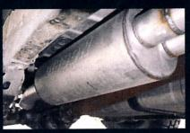
A Free-flowing headers don't help much if there's restrictive plumbing downstream. A Gibson muffler flows freely, is durable, and sounds great.
