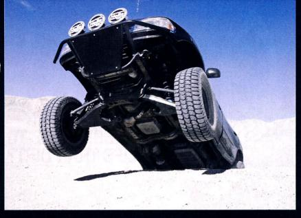
▶ If you opt to go the SUV route, it's a bit trickier to build a proper longtravel prerunner compared to building a pickup. The area around the rear door and quarter-panel stands in the way both in
