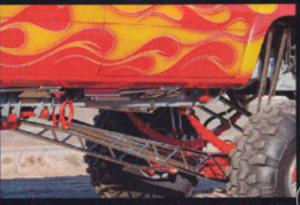
Front and year traction links were custom-made for this 3500 HD and thoroughly control front and year axie housing wap without inducing unwanted suspension bind, thanks to the trio of spherical bushing fitted to the pivot points of each link. Non-functional but good looking chrome plating from foss Plating draws the eye to the silick Fourst Engineering fabrication. Look close and you'll see a stabilists Given exhaust notices turked series just allowe the traction links.
