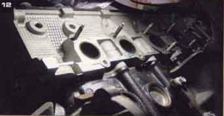
If carbon deposits and high spots appear on the head surface, use a scraper to remove them, being careful to not gouge the aluminum heads.
