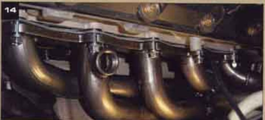
Now you're ready to install your new header. Gibeon recommends applying a small amount of hi-temperature sealer to the exhaust pipe flare before installing them. Some twisting and wiggle of the header is usually necessary. After installing the header, re-install the dipstick, then the EGR tube (if your truck had one). Repeat header installation on passenger side.
