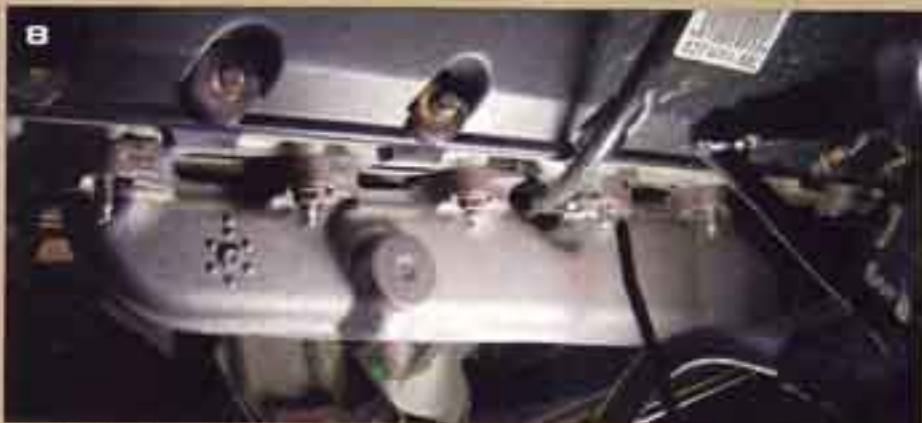
Now it's time to get rid of some unsightly dead weight. Remove the nuts attaching the manifold to the head. The nuts are on a stud, which also must be removed. If you end up removing both at the same time, congratulations! That is what you need to do anyway, but more often than not, you will remove the nut and then the stud separately.
