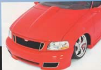
► The front edge of the hood was flared out where it meets the headlights, and a panel that closely resembles Garton's Speed Bumper was molded in. The windshield seal also had to be built from scratch, due to the new contour of the glass.
