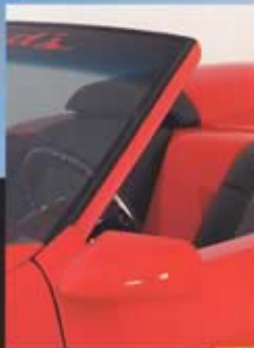
► Once the roof was cut off, the factory windshield was laid back 3 inches, which meant that the A-pillars had to be built from scratch. The doors were cut down 1 1/2 inches, so new door mounts for the Street Scene owners also had to be fabricated.
