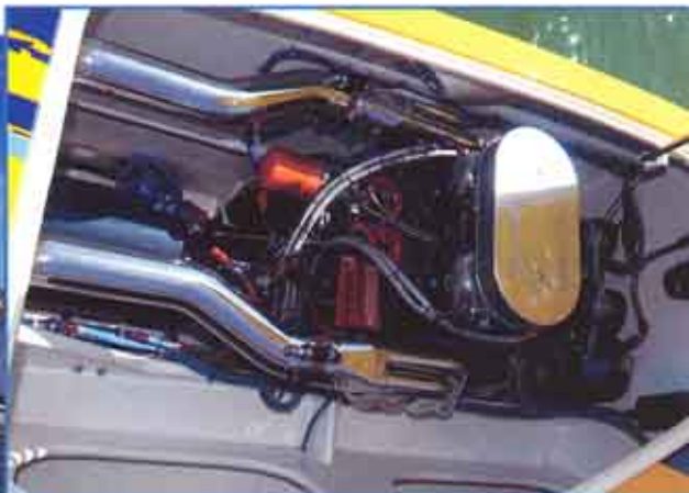
Twin 572 cubic inch engines dyno'ed at 1120 HP at 6000 rpm - on 91-octane pump gas.
