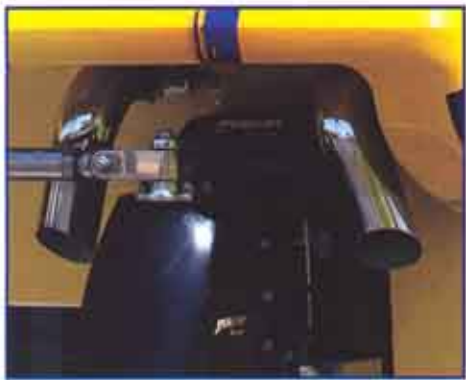
Custom designed exhaust tips send the exhaust below the water line at no-wake speeds - greatly reducing the sound volume.
