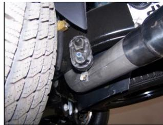
**5.** Next, install the exit pipes #D. Use clamp #F to secure to the tailpipe. DO NOT TIGHTEN. Insert welded hanger into rubber grommet.
