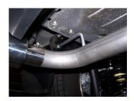
7. Install muffler assembly #E onto extension pipe. Insert hangers into rubber grommets. Use clamp #H to secure pipes together. Do not tighten.
