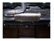
6. Install extension pipe #D onto extension pipe #C. Use clamp #H to secure pipes together. Do not tighten. Insert welded hanger into rubber grommet.
