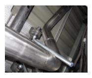
7. Install passenger side tailpipe #D into muffler 1.5-2". Insert welded hanger into rubber grommet. Use clamp #H to secure. Do not tighten. Install exit pipes #E onto tailpipes. Use clamps #H to secure pipes together. Do not tighten. Use zip ties to secure brake and fuel lines away from exhaust.
