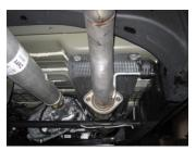
3. Install head pipe #A onto flange. Use your factory nuts.. Insert hanger into rubber grommet. Do not tighten. \*On short beds cut 12.5" off head pipe
