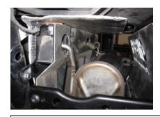
3. Next install the Gibson Muffler assembly. Install the bottom hanger mounts first then slide the inlet over the factory head pipe re using the factory gasket and springs.
