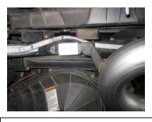
4. With the springs installed and the exhaust in the desired position mark the holes on the frame for the tailpipe hangers. You can either drill the holes and through bolt or use the provided self tapping screws.
