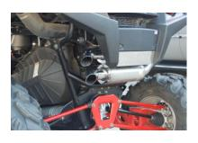
6. Install Item #A slide the hangers in factory mounts from the passenger side until lined up with the header. Once you have it lined up re install the
