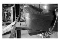
INSTALL YOUR STAINLESS STEEL TIP. USE ANY ALUMINUM OR STAINLESS STEEL CLEANER TO POLISH YOUR TIP. TIGHTEN ALL CLAMPS AND HANGERS. REINSTALL THE REAR SHOCK MOUNT.
