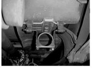
INSTALL HANGER #D INTO THE FACTORY RUBBER GROMMETS BEHIND THE MUFFLER LOCATION. THIS WILL HELP ALIGN THE MUFFLER AND HEADPIPE.
