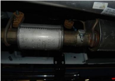
1. LAY OUT THE EXHAUST SYSTEM SO IT MATCHES THE DRAWING. MAKE SURE ALL PART NUMBERS ARE CORRECT. UNBOLT THE WELDED MUFFLER ASSEMBLY IN FRONT OF THE MUFFLER. **DO NOT REMOVE THE EXTENSION PIPE BEHIND THE CONVERTER.** FOR AN EASIER REMOVAL OF THE FACTORY EXHAUST. CUT THE TAILPIPE JUST BEHIND THE FACTORY MUFFLER. LEAVE ALL RUBBER GROMMETS IN PLACE. USE WD-40 FOR EASIER REMOVAL OF FACTORY HANGER.
