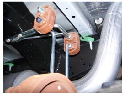
4. INSTALL OVERAXLE TAILPIPE # C INTO THE OUTLET OF THE MUFFLER 1 1/2" TO 2". INSERT THE REAR WELDED HANGER INTO THE FACTORY RUBBER GROMMET. USE CLAMP #E TO ATTACH THE OVERAXLE PIPE TO THE MUFFLER OUTLET. DO NOT TIGHTEN.
