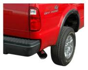
7. Install stainless steel tip. Make sure not to cover the louvers with the tip. The tip should come right up to the louvers, but do not cover. Clamp down. When you have everything in place, firmly tighten all bolts and clamps down securely. Use stainless steel cleaner and a Scotch Brite pad weekly to prevent tip from discoloration. Inspect all fasteners after 25-50 miles of operation and re-tighten as necessary. You may need to cut your stock tail pipe back to get your tip to fit correctly.
