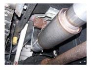
4. Install muffler #B onto headpipe #A 1.5"-2" with the louvers facing towards the tailpipe. Use clamp #G to secure the muffler to the headpipe. Do not tighten. Muffler outlet is looking into the louvers.
