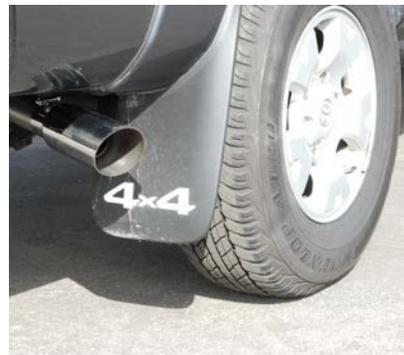
ALUMINUM OR STAINLESS STEEL CLEANER TO POLISH YOUR TIP. MAKE SURE YOU HAVE A MINIMUM OF A 1" CLEARANCE ON ALL PIPES FROM ALL RUBBER BRAKE LINES, TIRES, SHOCKS, FUEL LINES, ETC. THEN TIGHTEN ALL CLAMPS AND HANGERS
