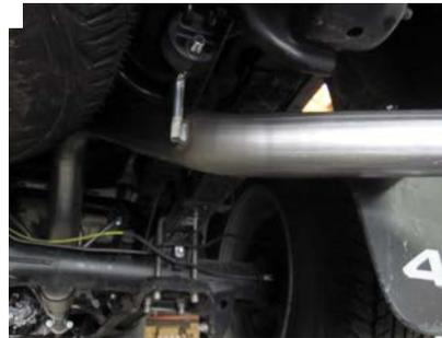
INSTALL MUFFLER #B ONTO HEAD PIPE 1-1/2" TO 2" WITH THE LOUVERS FACING TOWARDS THE CONVERTER. THE MUFFLER OUTLET SHOULD BE POSITIONED AT 12:00. USE A JACK STAND TO SUPPORT THE MUFFLER. USE CLAMP #E TO SECURE THE MUFFLER TO THE HEAD PIPE. DO NOT TIGHTEN. MUFFLER INLET IS LOOKING INTO THE LOUVERS.
