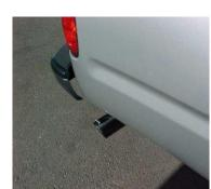
**NEXT INSTALL YOUR** STAINLESS STEEL TIP TO YOUR DESIRED LOOK, USE ANY ALUMINMUM OR STAINLESS STEEL CLEANER TO POLISH YOUR TIP. MAKE SURE YOU HAVE A MINIMUM OF A 1" CLEARANCE ON ALL PIPES FROM ALL RUBBER BRAKE LINES, TIRES, SHOCKS, FUEL LINES, ETC. THEN TIGHTEN ALL CLAMPS AND **HANGERS**
