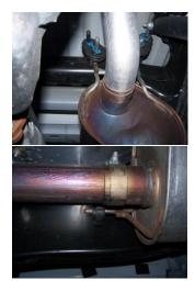
1. To remove the stock exhaust un-clamp it just behind the stock muffler. Then un-clamp stock muffler and remove. Leave all rubber grommets in place. Use WD-40 to aid in removal of exhaust.
