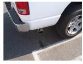
**6.** Install stainless steel tip #D. Clamp down. When you have everything in place, firmly tighten all bolts and clamps down securely. Use stainless steel cleaner and a Scotch Brite pad weekly to prevent tip from discoloration.
