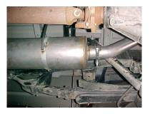
SLIDE BAND CLAMP #G ONTO MUFFLER #B. INSERT HANGERS INTO RUBBER GROMMETS. USE BOLT KIT #H TO TIGHTEN UP BAND CLAMP.
