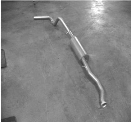
TO REMOVE EXHAUST UNBOLT THE 2 BOLT FLANGE LOCATED JUST BEHIND THE CATALYTIC CONVERTER. **YOU WILL RE-USE STOCK FLANGE BOLTS.** NOW CUT OFF YOUR STOCK TAILPIPE JUST BEHIND THE MUFFLER AND REMOVE. LEAVE ALL RUBBER GROMMETS ON THE HANGER. USE WD-40 TO AID IN THE REMOVAL OF EXHAUST AND HANGERS.
