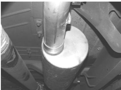
INSTALL MUFFLER #B ONTO HEADPIPE 1-1/2" TO 2" WITH INLET TOWARDS THE MOTOR. OUTLET SHOULD BE AT THE 9 O'CLOCK POSITION USE CLAMP #F TO SECURE MUFFLER TO THE HEADPIPE. USE A JACKSTAND TO SUPPORT MUFFLER. DO NOT TIGHTEN. MUFFLER INLET IS LOOKING INTO LOUVERS.
