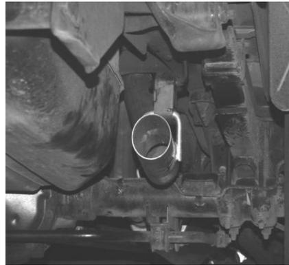
SLIDE TAILPIPE #C INTO MUFFLER 1-1/2" TO 2". INSERT WELDED HANGER INTO RUBBER GROMMETS USING CLAMP #F TO SECURE TAILPIPE TO MUFFLER. DO NOT TIGHTEN.
