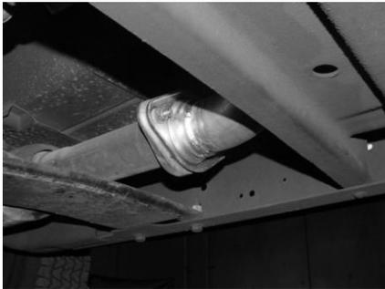
BOLT HEADPIPE #A ONTO STOCK FLANGE RE-USING STOCK BOLTS. INSERT WELDED HANGER INTO RUBBER GROMMET.
