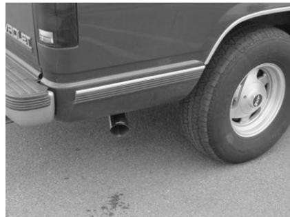
INSTALL YOUR STAINLESS TIP NOW, TIGHTEN ALL NUTS, BOLTS, CLAMPS AND FLANGE STARTING FROM THE HEADPIPE AND WORK YOUR WAY BACK.
