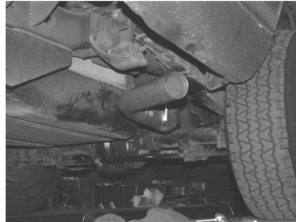
SLIDE TURNOUT PIPE #D ONTO TAILPIPE 1 1/2" TO 2". YOU MAY HAVE TO TRIM THE END OF THE PIPE FOR PROPER LENGTH FOR YOUR VEHICLE. USE CLAMP #F TO SECURE PIPE TO TAILPIPE.
