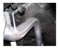
NEXT, INSTALL OVERAXLE TAILPIPE # D INTO MUFFLER 1-1/2"- 2". USE CLAMP # I TO SECURE PIPE TO MUFFLER, DO NOT TIGHTEN. INSERT HANGER INTO RUBBER GROMMET.
