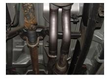
SLIDE PASSENGER SIDE HEADPIPE #A ONTO STOCK HEADPIPE. INSERT WELDED HANGER INTO RUBBER GROMMET. NEXT, INSTALL DRIVERS SIDE HEADPIPE #B ONTO STOCK HEADPIPE, USE CLAMP #H TO SECURE BOTH HEADPIPES, DO NOT TIGHTEN.
