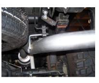
SLIDE EXIT PIPE # E ONTO OVERAXLE TAILPIPE INSERT WELDED HANGER INTO RUBBER GROMMET. USE CLAMP # I TO SECURE PIPES TOGETHER. DO NOT TIGHTEN. ROTATE PIPE UNTIL LEVEL.
