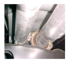
REMOVE YOUR STOCK EXHAUST FROM THE FACTORY FLANGES LOCATED JUST BEHIND YOUR FACTORY Y-PIPE, NEXT CUT OFF YOUR TAILPIPE JUST BEHIND THE MUFFLER. USE WD-40 TO AID IN REMOVAL OF RUBBER GROMMETS FROM HANGERS.
