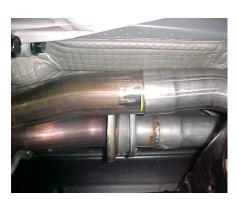
INSTALL PASS. SIDE HEADPIPE # A ONTO FACTORY FLANGE USING THE HARDWARE # H. INSERT WELDED HANGER INTO RUBBER GROMMET. DO NOT TIGHTEN. NEXT INSTALL DR. SIDE HEADPIPE # B ONTO FACTORY PIPE USE CLAMP # F TO SECURE, DO NOT TIGHTEN.
