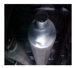
INSTALL MUFFLER # C ONTO HEADPIPES 1 ½"-2". USE CLAMPS # F TO SECURE OUTLET OF MUFFLER, IT SHOULD BE AT THE 12 O'CLOCK POSITION. USE A JACKSTAND TO SUPPORT MUFFLER.
