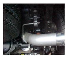
INSTALL OVER-AXLE TAILPIPE # D INTO MUFFLER 1 <sup>1</sup>/<sub>2</sub>" – 2", INSERT WELDED HANGER INTO RUBBER GROMMET, ROTATE PIPE TO PROPER ANGLE.
