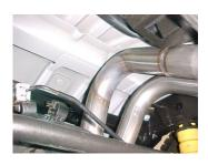
4. Slide driver side over axle tailpipe #B into muffler 1.5-2". Use clamp #F to secure tailpipe to muffler. Do not tighten. Insert welded hanger into rubber grommet.
