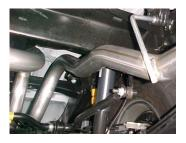
6. Slide the passenger side tailpipe #D into muffler 1.5-2". Insert welded hanger into rubber grommet. Use clamp #F to secure tailpipe to muffler. Do not tighten.
