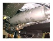
3. Slide muffler #A onto headpipe 1½"-2". Use a jack stand to support the muffler. Make sure muffler outlets are level. Use clamp #G to secure the muffler to the headpipe. Do not tighten.
