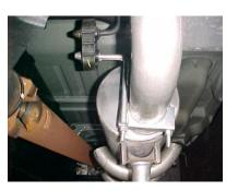
Install muffler #C onto head pipes B 1-1/2" to 2"with the louvers facing towards the converter. Use a jack stand to support the muffler. Use clamps #G to secure the muffler to the head pipes. Do not tighten. Outlet of muffler should be at 6 o'clock.
