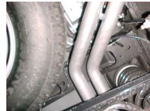
Install drivers side overaxle tailpipe #D onto front tailpipe. Use clamp #I to secure together. Do not tighten. Use bolt kit #L to secure pipes together. Tab on drivers' side tailpipe will be on top.
