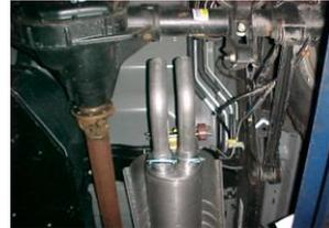
Install the passenger side front tailpipe #E  $1\frac{1}{2}$ " to 2" into muffler. Use clamp # H to secure front tailpipe to muffler, and attach hanger # K. Do not tighten.
