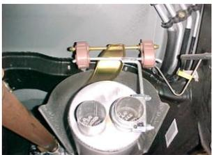
Install rear muffler T-hanger #K into rubber grommets located just above the muffler outlets. Shorter side of the hanger will be inserted on the passenger side grommet. Slide clamp onto passenger side muffler outlet. Do not tighten.
