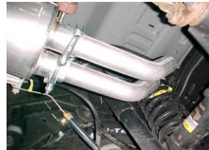
Install drivers side front tailpipe #C into muffler  $1\frac{1}{2}$ " to 2". Use clamp #H to secure front tailpipe to muffler. Do not tighten.
