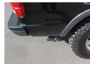
Install the stainless steel tips. Clamp down. To clean your stainless tips, use a scotch brite pad and any stainless steel or aluminum cleaner. Now go back and tighten all clamps, nuts and bolts. Start from the front and work back.
