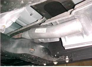
Install head pipe #A onto your existing stock front pipe and secure with clamp #H. Use a jack stand to support the converter. Do not tighten.
