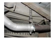
INSTALL HANGER #H ON REAR PASSENGER AND DRIVER SIDE FRAME RAIL 4" BACK AND 4" UP FROM YOUR STOCK HANGER, USE THE BOLT KIT PROVIDED AND USE THE 2<sup>ND</sup> HOLE FROM THE TOP OF THE 10" HANGER.
