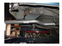
**INSTALL PASSENGER SIDE** OVERAXLE TAILPIPE #C INTO OUTLET OF MUFFLER. USE CLAMP #I TO SECURE, CLAMP AND SECURE THE REAR OF THE TAILPIPE TO HANGER #H USING CLAMP #I. INSTALL FRONT DRIVERSIDE OVERAXLE TAILPIPE #D AND SECURE TO MUFFLER USING CLAMP #G. **INSTALL REAR TAILPIPE #E AND SECURE TO** FRONT TAILPIPE USING CLAMP #I. CLAMP AND SECURE THE REAR OF THE TAILPIPE TO HANGER #H USING CLAMP #I. DO NOT TIGHTEN.
