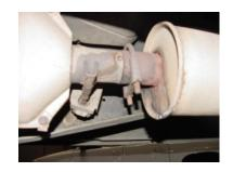
REMOVE YOUR STOCK EXHAUST BY UN-CLAMPING YOUR MUFFLER RIGHT BEHIND THE CATALYTIC CONVERTER. LEAVE ALL RUBBER GROMMETS IN PLACE. USE WD-40 TO AID IN THE REMOVAL OF YOUR STOCK EXHAUST.
