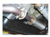
TO REMOVE YOUR STOCK EXHAUST, REMOVE IT FROM THE 2-BOLT FLANGE LOCATED JUST IN FRONT OF THE MUFFLER REMOVE HANGERS FROM RUBBER GROMMETS BY PULLING EXHAUST TOWARDS THE REAR OF THE VEHICLE, USE WD-40 TO AID IN REMOVAL, LEAVE GROMMETS IN PLACE.
