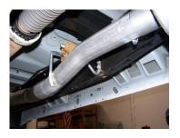
INSTALL HEADPIPE # A ONTO FACTORY PIPE. LINE UP THE NOTCH. USE CLAMP # G TO SECURE HEADPIPE TO FACTORY PIPE. DO NOT TIGHTEN. INSERT WELDED HANGER INTO RUBBER GROMMET.
