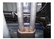
4. Install muffler #C onto headpipes 1.5"-2" with the louvers facing towards the converter. Use a jack stand to support the muffler. Use clamps #J to secure the muffler to the headpipes. Do not tighten. Muffler inlet is looking into the louvers.
