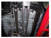
3. Install passenger side headpipe #A using your stock bolts. Do not tighten. Next, install driver side headpipe #B using stock bolts. Do not tighten. Install metal hangers into rubber grommets.
