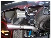
7. Install rear tailpipe hanger #K. Use bolt kit #L to secure. Use the hole on frame closest to the rear shackle. Install rubber grommet on rear hanger.
