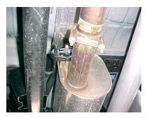
YOU MAY NEED TO HEAT IT UP FOR EASIER REMOVAL. LEAVE ALL RUBBER GROMMETS IN PLACE. USE WD-40 FOR REMOVAL OF HANGERS. FOR EASIER REMOVAL, REMOVE THE TWO CROSSMEMBER BARS FIRST.
