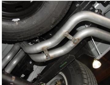
INSTALL PASSENGER SIDE TAILPIPE #D INTO MUFFLER AND ATTACH USING CLAMP #F. INSERT WELDED HANGER INTO RUBBER GROMMET. DO NOT TIGHTEN. USE BOLT KIT #I TO ATTACH THE TAILPIPES TOGETHER. DO NOT TIGHTEN. PASSANGER SIDE TABS ON THE TAILPIPE WILL BE ON TOP OF THE DRIVERSIDE TABS.
