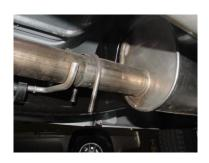
TO REMOVE STOCK **EXHAUST UNCLAMP** THE STOCK EXHAUST **JUST IN FRONT OF THE MUFFLER.** YOU MAY NEED TO HEAT IT UP FOR EASIER REMOVAL. LEAVE ALL RUBBER GROMMETS IN PLACE. USE WD-40 FOR REMOVAL OF HANGERS.
