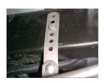
MEASURE 19 1/2" FROM THE REAR OF THE FRAME AND USE THIS HOLE AND BOLT ON HANGER # F. USE THE 3<sup>RD</sup> HOLE FROM THE TOP.
