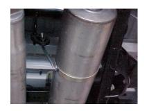
INSTALL MUFFLER #B ONTO HEADPIPE #A 1-1/2" TO 2". USE CLAMP #H TO SECURE THE MUFFLER TO THE HEADPIPE. DO NOT TIGHTEN. SLIDE BAND CLAMP #I ONTO THE MUFFLER AND INSERT THE WELDED HANGER INTO THE RUBBER GROMMET. ATTACH WITH BOLT KIT # K.
