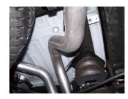
5. Slide the over axle tailpipe #C into the muffler 1.5-2". Use clamp #E to secure tailpipe to muffler. Do not tighten. Insert welded hangers into rubber arommets.
