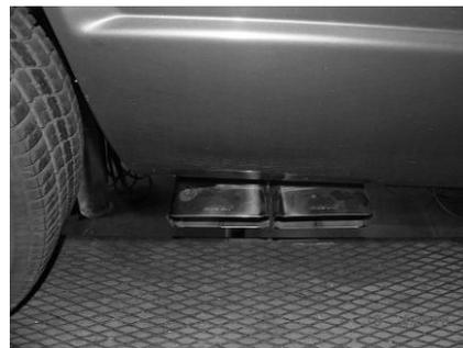
**MAKE SURE YOU HAVE A 1" CLEARANCE ON ALL PIPES FROM ALL BRAKE, FUEL LINES, SHOCKS, TIRES, ETC...**
