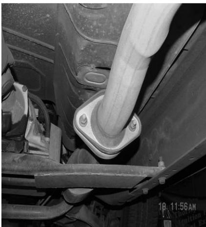
TO REMOVE EXHAUST- UNBOLT THE FLANGE LOCATED BEHIND THE CATALYTIC CONVERTER. **SAVE STOCK NUTS AND BOLTS FOR YOU WILL REUSE THEM.** NOW CUT OFF YOUR STOCK TAILPIPE JUST BEHIND THE MUFFLER AND REMOVE. LEAVE ALL RUBBER GROMMETS ON THE HANGER. USE WD-40 TO AID IN THE REMOVAL OF THE EXHAUST AND HANGERS.
