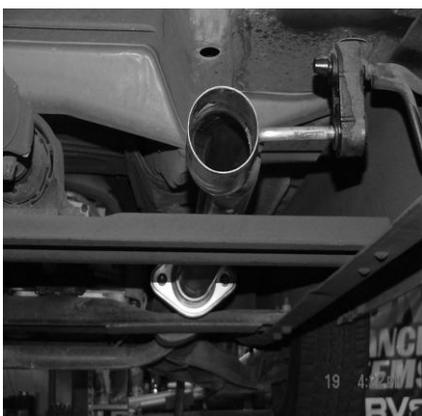
BOLT HEADPIPE #A TO STOCK FLANGE USING GASKET # F AND RE-USING STOCK NUTS AND BOLTS. INSERT WELDED HANGER INTO RUBBER GROMMETS.
