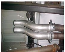
SLIDE PASSENGER SIDE HEADPIPE #A ONTO STOCK HEADPIPE. INSERT WELDED HANGER INTO RUBBER GROMMET. NEXT INSTALL DRIVERS SIDE HEADPIPE #B ONTO STOCK HEADPIPE, USE CLAMP #G TO SECURE HEADPIPES, DO NOT TIGHTEN.
