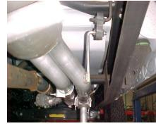
SLIDE DRIVERS SIDE TAILPIPE #D INTO MUFFLER 1-1/2" TO 2". INSERT WELDED HANGER INTO RUBBER GROMMET AND ATTACH TO MUFFLER USING CLAMP #H. THE PASSENGER SIDE TAILPIPE WILL BE ON THE BOTTOM.
