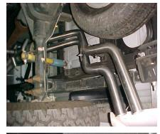
ATTACH BOTH TAILPIPES TOGETHER WITH BOLT KIT #J.
