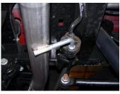
5. Slide the second driver side over axle tailpipe #C onto pipe #B 1.5-2". Secure pipes using clamp #F. Do not tighten. Insert welded hanger into rubber grommet.
