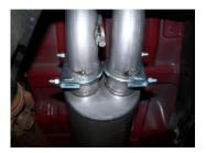
6. Slide the passenger side tailpipe #D into muffler 1.5-2". Insert welded hanger into rubber grommet. Use clamp #F to secure tailpipe to muffler. Do not tighten.
