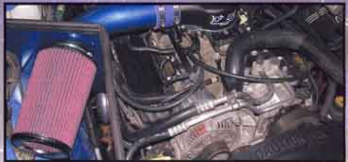
The 5.2-liter V-8 features an F88 throttle body, Gibson headers and a 360 Degree Air Intakez intake system.
