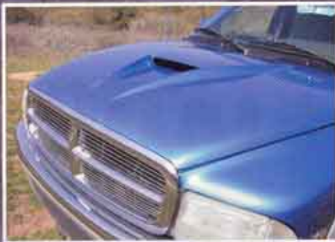
Flickinger replaced the factory steel hood with a fiberglass Cervinis hood.
