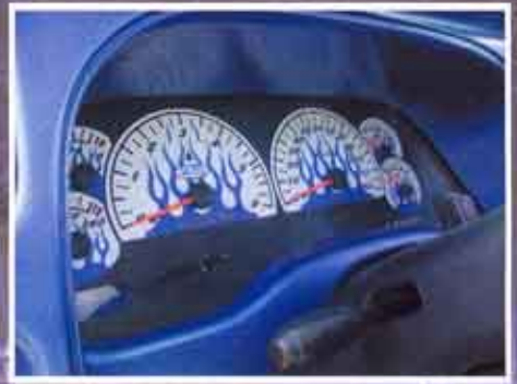
The factory gauges were replaced with Nu Image flamed face gauges. A Nu Image AC face panel is also used.
