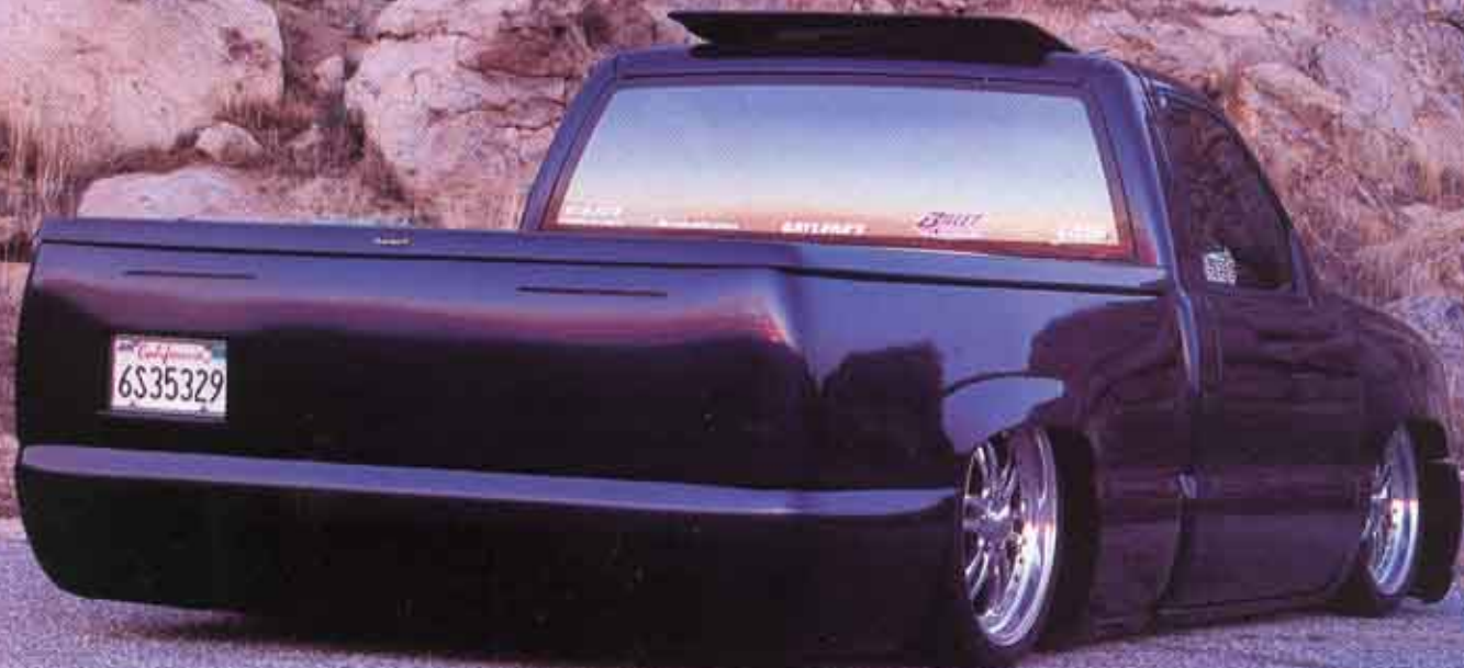
Jon welded his tailgate shut and then frenched a set of LED taillights into the tailgate along with the license plate setup. The Sir Michaels roll pan finishes off the elegance.
