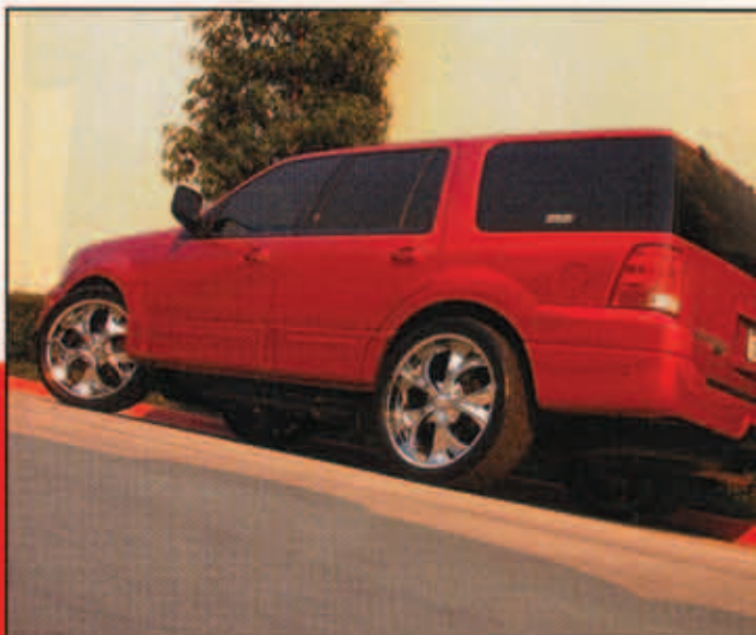
The lowered stance came from taking the SUV to Advantage Performance where some coil spring work was done to lower the Expedition two inches.
