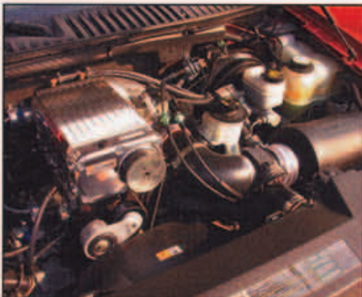
The twin-screw supercharger system on this SUV is responsible for pushing out 386 horsepower out of the 5.4-liter V-8.
